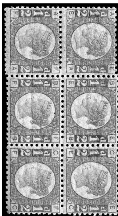
Fig. 21.5 Effect of inverted feed on location of broken perforation pins. Broken pins 2-4 on stamp RH indicate normal top feed; pins 10-12 on stamp ME confirm inverted feed; both stamps are from Plate 9 (SG Spec G2)
