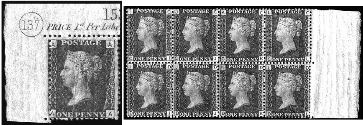
Figs. 21.1 and 21.2 Stamps showing effect of broken horizontal and vertical pins, the latter between columns I and J and both sides of marginal column L. Both show extension holes in their side margins
