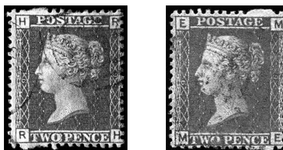
Fig. 21.5 Effect of inverted feed on location of broken perforation pins. Broken pins 2-4 on stamp RH indicate normal top feed; pins 10-12 on stamp ME confirm inverted feed; both stamps are from Plate 9 (SG Spec G2)
